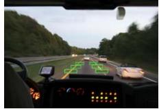
Iteris' LDW system works effectively both day and night and in most weather conditions where lane marks are visible. Truck drivers say it is a big help in fog, rain and other low visibility conditions. The LDW system warns drivers of these unintentional drifts anywhere there are lane markings. It will warn on the shoulder-line, centerline and between lanes, and picks up both solid and dashed lines; even if the lines are heavily faded.
